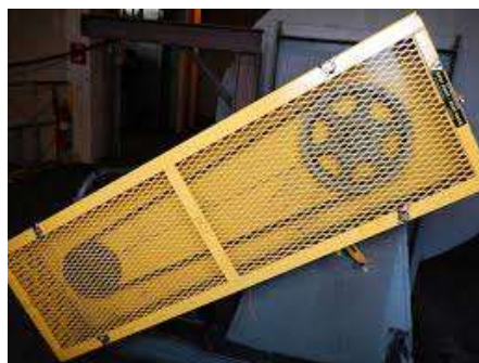
Figure 25 –SHOWING A SUITABLE GUARD FOR A BELT DRIVE
