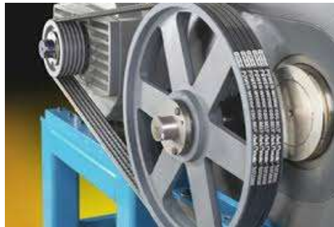
Figure 19 – SHOWING A TYPICAL V-RIBBED BELT INSTALLATION.
