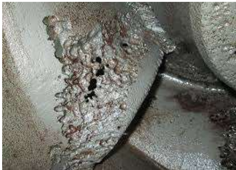
Figure 30 – SHOWING DAMAGE TO AN IMPELLER CAUSED BY CAVITATION.
