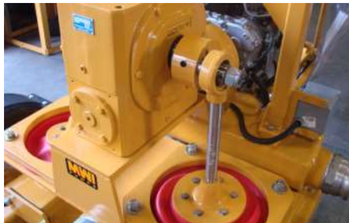
Figure 19 – A TYPICAL CONSTRUCTION SITE DEWATERING DIAPHRAGM PUMP.
