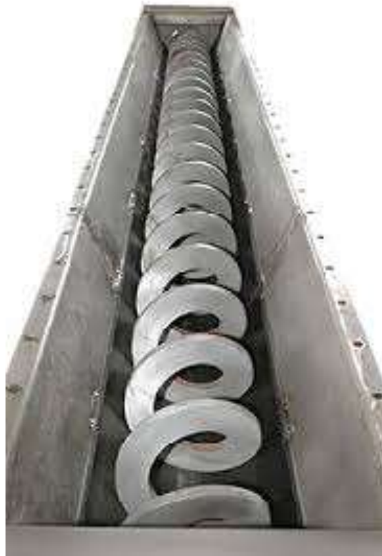
Figure 25 – AN EXAMPLE OF A SHAFTLESS SCREW CONVEYOR.
