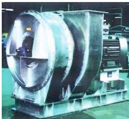
Figure 51 – SHOWING A TYPICAL TWO-STAGE CENTRIFUGAL BLOWER.
