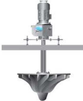
Figure 32 – EXAMPLE OF VERTICAL SHAFT SURFACE AERATOR.
